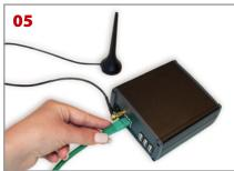
Plug-in a RJ45 ethernet cable.
