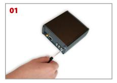
Open the FOXBOX case removing all the Insert the SIM card in the placeholder. screws. Extract the electronic inside.
