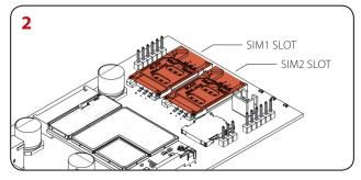
Insert the SIM card into the "SIM1" slot.
