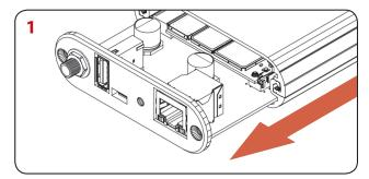
Pull out the rear panel and the board from the case.
