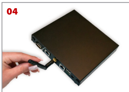
04 Plug-in the antenna connector.
