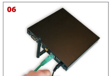
06 Plug-in the power supply.
