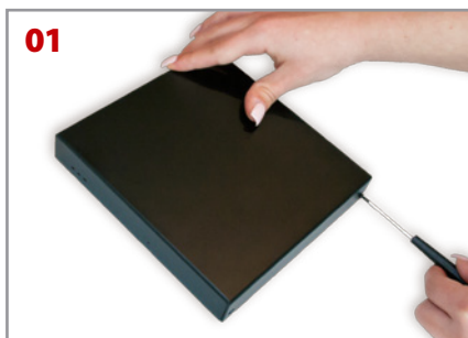
01 Open the FOXBOX case removing all the screws. Extract the electronic inside.
