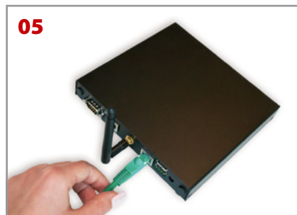
05 Plug-in a RJ45 ethernet cable.
