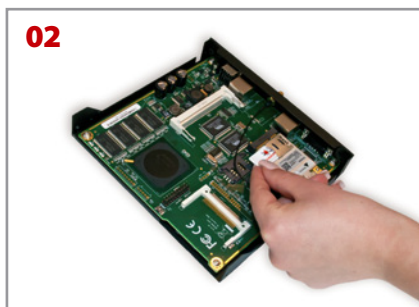
02 Insert the SIM card in the placeholder.
